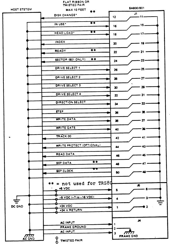
NOTE. Not shown are 6 of the 9 Alternate I/O connections. The connections for these lines are on pins 2, 4, 6, 8, 10, and 14 Signal return for these lines are on pins 1, 3, 5, 7, 9 and 13 respectively. Reference section 7 for uses of
